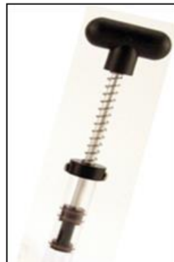
Stemple pipette for taking A measured amount of a Plankton sample for counting
