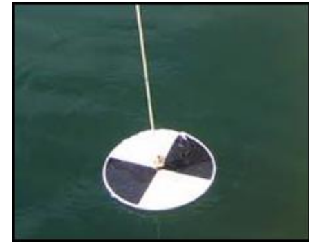
Sechii disk used to measure the depth that line penetrates the water. The disk is lowered until it disappears and the deep of disappearance is measure from markings on the lowering line.
