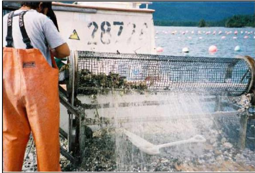
Tumbler/washer that cleans and removes fouling from oyster and also helps the oyster grow more meat.
