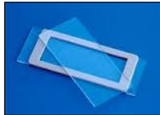
Plankton counting chamber that holds 1 to 5 mls. of sample
