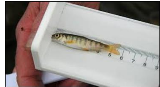
Fish measuring board used In fish hatchery and by field Biologist to rapidly measure fish and prevent abrasion of the fish's skin
