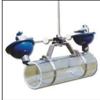
Van Dorn water sample for taking water samples under the water surface
