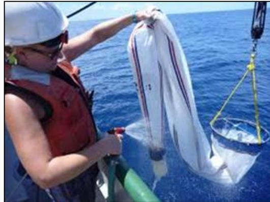
In this example, the sample volume of 500 ml collected by the plankton net. Five samples 1 ml in volume will be drawn out of this sample with a Stemple pipet for counting.
