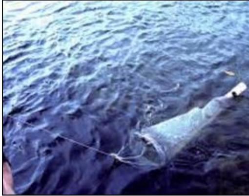
Washing the captured sampling into the cod end chamber The net is lifted out of the water and the sides are washed to capture the plankton sample into the cod end chamber.
